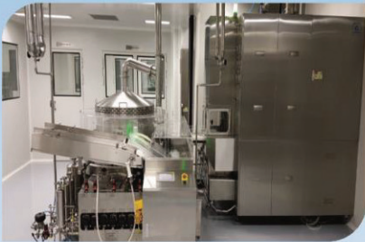
Ampoule Washing Machine with ultrasonic Ampoule Depyrogenizing Tunnel Capacity : 22,500,000 ampoules/year
